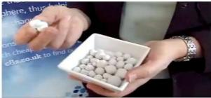
Above: The Carbon 8 process by which the hazardous APCr ash residue is turned ito small balls which can then be safely re-used and not have to be expensively buried in lined ash pits.
